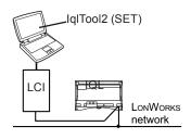
IqITool2 facilitates mapping the LonWorks segment, resolving duplicate addresses on the LonWorks network, water balancing (/WR2, /WR4, /WT2, /WT4 only), identifying using service button, associating with SDU-LON, monitoring inputs and exercising outputs, setting as a timekeeper, and configuring for RD. It provides access to text communications for changing module parameters (e.g. knobs, switches, changing a generic strategy).
