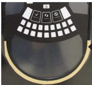
Figure 3: Remove Backing to Stick Cover Down
