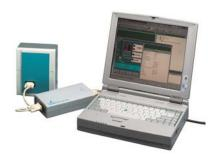
The PC - Link High Level Interface (PC - Link HLI) connects a PC and VESDA system. Each PC - Link HLI includes two cables (It does not include a PC):
