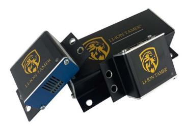
The Li-ion Tamer GEN 3 is a device that detects the venting of battery electrolyte solvent vapours (off-gassing phase) that occurs early in the failure mode of lithium-ion batteries (LIB). The early detection of this event allows proper mitigation steps to be taken to avoid a catastrophic thermal runaway failure.
